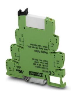
PLC relay, consisting of base terminal block PLC-BSP.../21 with spring-cage connection and pluggable miniature relay with power contact, for assembly on mounting rail NS 35/7.5, 1 PDT, input voltage 12 V DC
